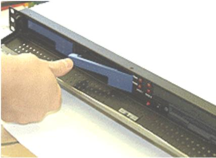
2. Use thumb to push the handle bar into the bay until the tray is firmly seated.
