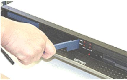
3. Grab the disk tray handle bar and pullout the disk unit out of the drive bay. Done.
