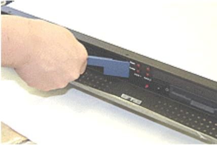
1. Slowly slide the hard disk tray into the server's drive bay. Grab the handle bar and slowly insert the hard disk tray unit into the server drive bay.
